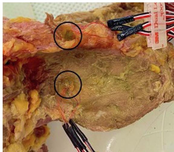
**Figure 1** Specimen demonstrating the positions of strain rosettes on the scapular spine and acromion. Black circles (○) demonstrate location of rosettes where strain was measured.
