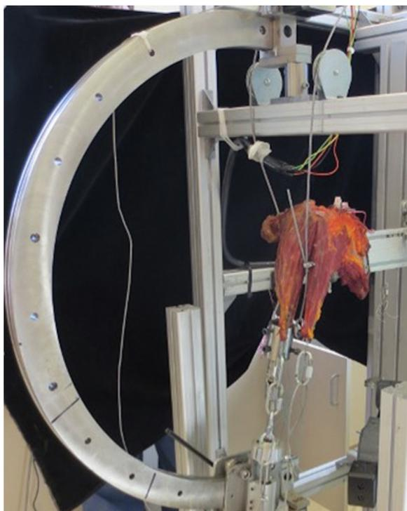
**Figure 2** Specimen on the custom dynamic shoulder frame. No. 5 ethibond was passed through two deltoid heads and loops were tied to connect to the pulley system that loaded the deltoid. The specimen was manually abducted to 30° and 60° and the humerus was then held at those angles.
